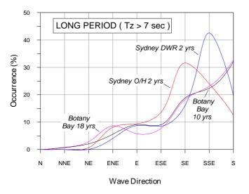
Figure 5 Wave Direction Distributions - Tz greater than 7s
