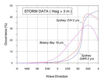
Figure 3 Wave Direction Distributions - Storm Data
